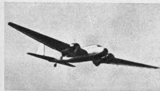
Wing dihedral, straight flat tailplane and non-retractable tailwheel are visible on Nell (above). As on the B-25, its two engines are underslung.
